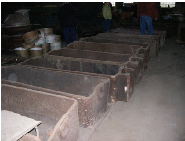
Tubs for charging furnaces
