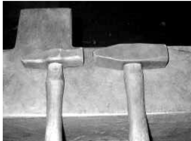
6. Use a smaller hammer to do this operation. The hammer on the left is a one-pound hammer— a good hammer weight for the task. The hammer on the right is a 1.8 pound hammer which is too heavy for this form.
