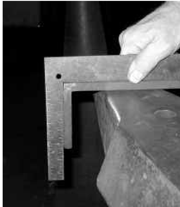
8. Check your work with a square. Note that the legs are square, but there is a gap near the corner of the long leg, which should be corrected.
