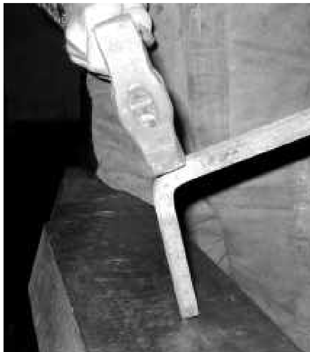
4. Vertical blow— note the position of the hammer and the short leg.
