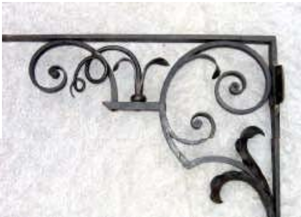
1. Shelf bracket made by Peter Ross. The snub end scrolls were made by making a very long ribbon taper, then tightly rolling the taper to form the snub end. This method of forging snub end scrolls was typical of English 18th century ironwork.
