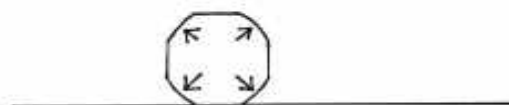
3. The remnants of the four original faces of the bar are shown bulged by the displacement of the metal as the corners are forged.
