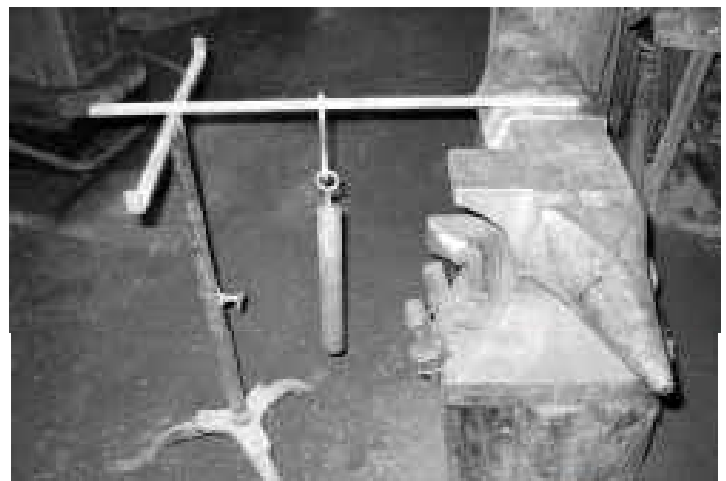
7. A blacksmith's helper stand helps to hold longer bars. The attached weight helps keep the workpiece steady. Adjust the blacksmith's helper so the workpiece lies flat on the anvil or cutting saddle.
