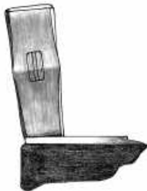
2a. The hammer head is tilted so the peen strikes the bar at the angle of the desired taper.
