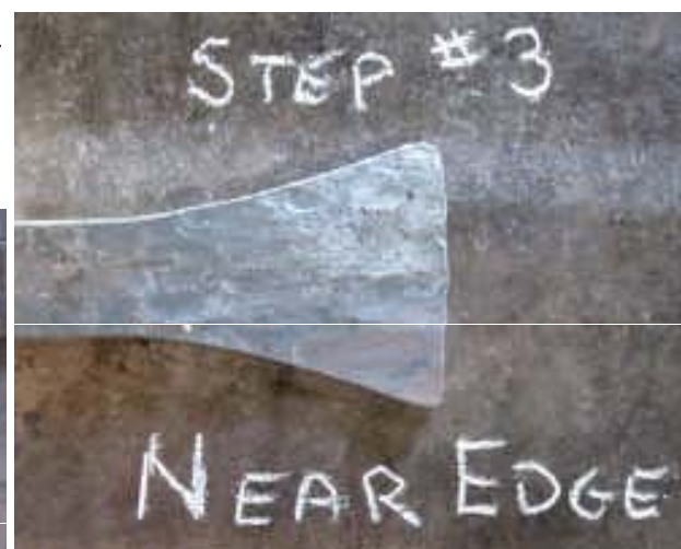
5. Both corners have been peened out in this photo. This is what the fishtail should look like before refining with the face of the hammer.
