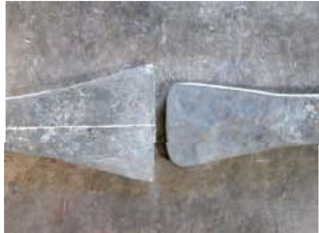
9. The forging on the right was made using only the hammer's face. It has the same taper and end thickness as this lesson's forging on the left, but could not achieve the desired width without sacrificing the other two dimensions
