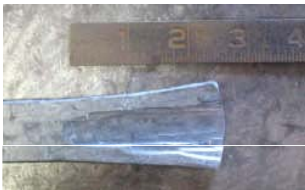
3. Centered trough formed by cross peen, 2 1/2" long.
