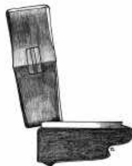
2b. Because the bar is held even with the far edge of the anvil, the corner of the hammer peen should never come in contact with the face of the anvil even if the blow lands a little wide of the mark. Working at a slightly rounded edge will prevent damage to the squarest edge of the anvil, should the bar slip back from the edge.
