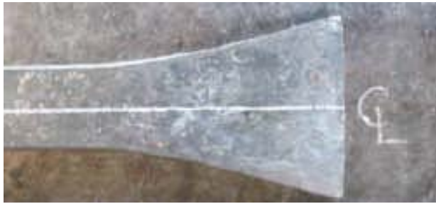
8. The refined fishtail shape. Note that the centerline of the parent bar is centered also in the fishtail.
