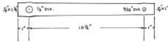
2. Flat bar in its unbent layout.
