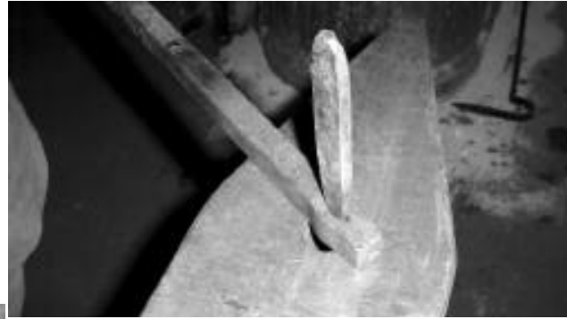
Supporting the bar with the edges of the pritchel hole
