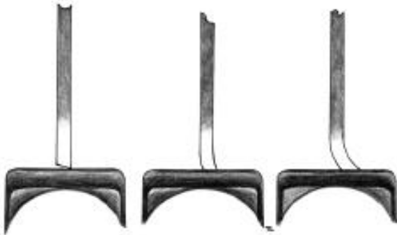
A bar end that is out of square causes bending
