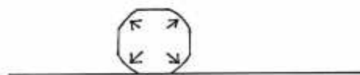
3. The remnants of the four original faces of the bar are shown bulged by the displacement of the metal as the corners are forged.
