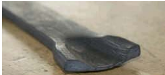
Fig. 10. Top of the bar showing peened middle trough.
