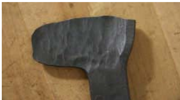
Fig. 14. Top view of the bar with one half spread.
