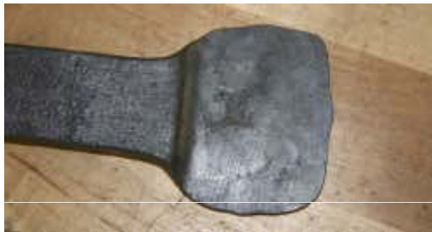
Fig. 17. Flattened bar using the face of the hammer
