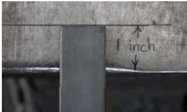
Fig. 5. One inch of the bar on the anvil face.
