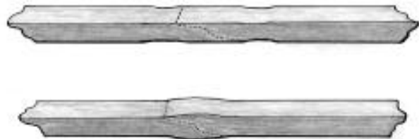
Figure 14: Top—thin areas due to loss of material from burning, too little upset, or over-hammering, must be upset. Bottom—remaining bulge must be drawn down to dimension.
