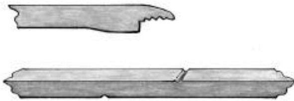
Figure 8: Blunt scarf makes seam difficult to blend.
