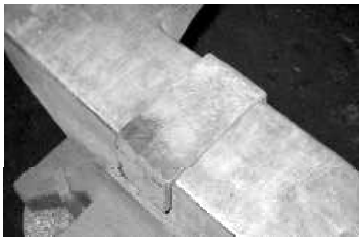
9. This cutting saddle was made from 1/2"x 3," lies flat on the anvil face and fits snugly over the edges. The thickness has been reduced by re-dressing the surface to eliminate surface scars made from cutting through the workpiece.'blacksmith's helper so the workpiece lies flat on the anvil or cutting saddle.
