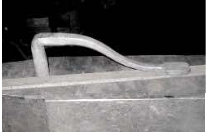
6. The holdfast slides into the pritchel hole, and holds the work-piece firmly with a light tap of the hammer above the holdfast's vertical shank. To remove the holdfast, lightly tap the side of tool's vertical shank with the hammer.
