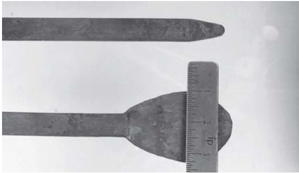
A water leaf blank from the scroll stock \frac{3}{4} -inch wide by \frac{1}{4} -inch thick to be folded back and welded to the scroll
