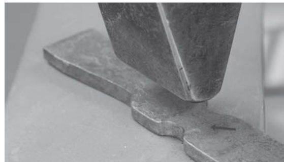
The side fullered material does not allow for clearance of the peen when spreading
