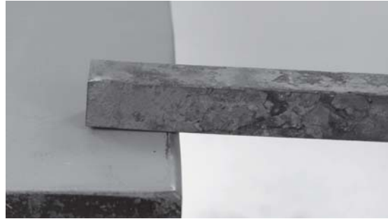
A \frac{3}{4} " square bar to be used to make a pair of tongs, about to be set down to half its thickness
