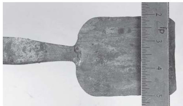
My result on spreading the 1-inch thick by 1/4-inch wide bar
