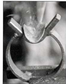
Scooping the leaf in a 45° swage designed to be used in a vise.
