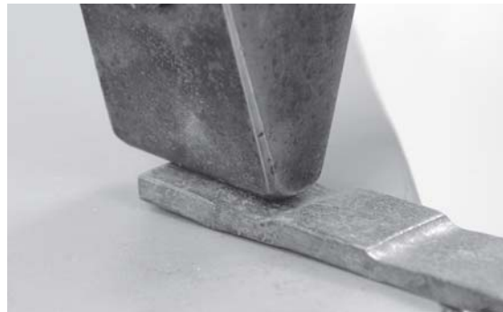
The set-downs on the face of the material allow clearance for the peen when spreading
