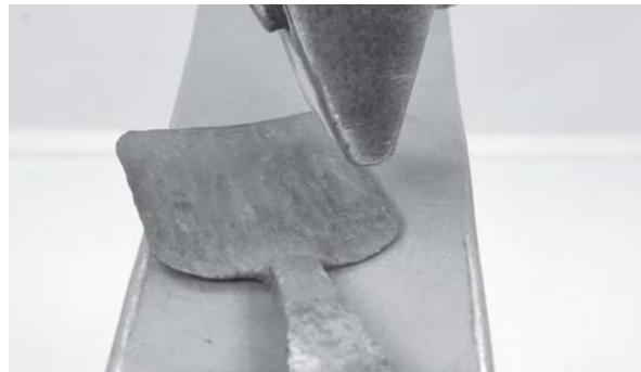
Spreading the 1-inch thick by 1/4-inch wide bar
