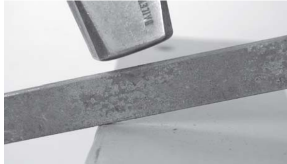
Necking in at the edge of the anvil with the hammer prior to spreading the material
