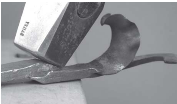
The water leaf and tip the scroll applied to the remainder of the scroll stock
