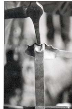
Scooping the leaf in a 45° swage designed to be used in a vise.
