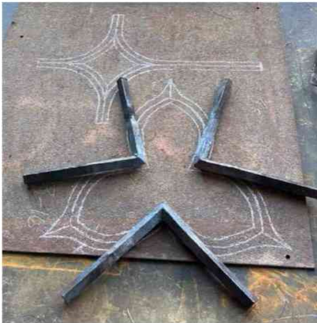
Below: Three right angles on the layout table before bending.
