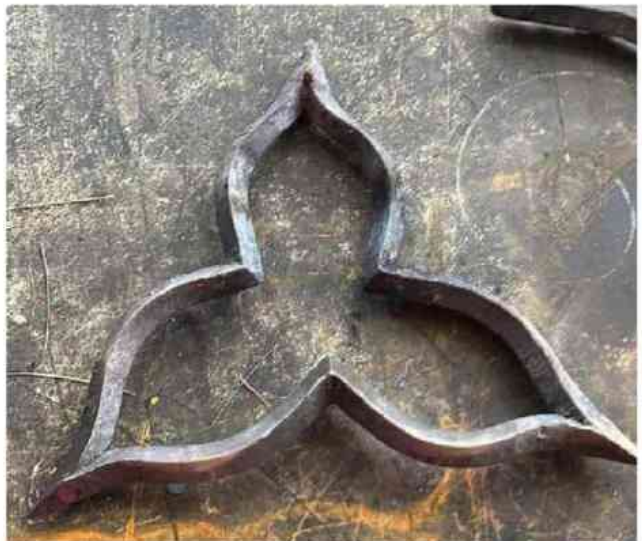
Below: The trefoil with the corners welded and forged to clean points with facets and corners neatly centered.
