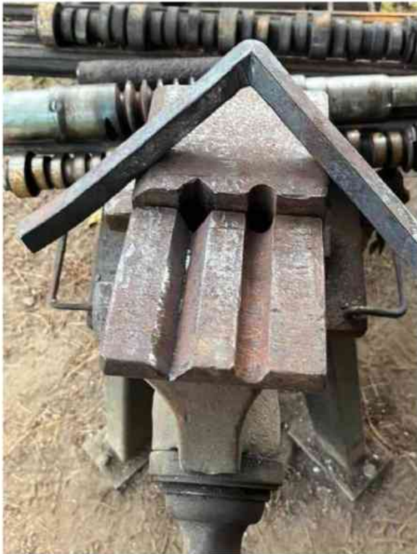
Above: Tooling for forming right angle on the diamond, set up in a vise.
