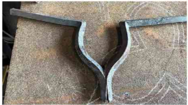
Above: two legs of the right angles bent and the ends flattened and fitted for welding. John bent and fitted all three lobes of the trefoil before welding.
